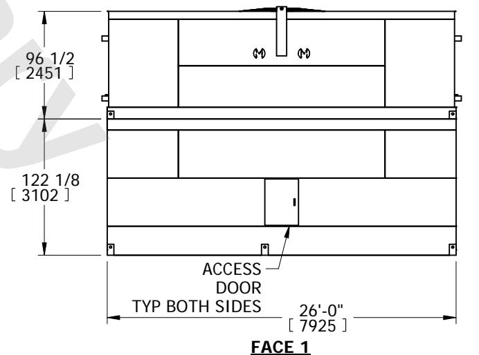
SHIPPING WEIGHT 71180 lbs+ [32290] kg+ OPERATING WEIGHT 112540 lbs+ [51050] kg+ HEAVIEST SECTION WEIGHT 24090 lbs+ [10930] kg+ NO. OF SHIPPING SECTIONS 4 DRAWN BY: TLS
