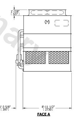
DRAWN BY: SLR NO. OF SHIPPING SECTIONS **SHIPPING** OPERATING HEAVIEST SECTION 12400 lbs+ [5625] kg+ 8030 lbs+ [3645] kg+ 9470 lbs+ [4300] kg+ WEIGHT WEIGHT WEIGHT
