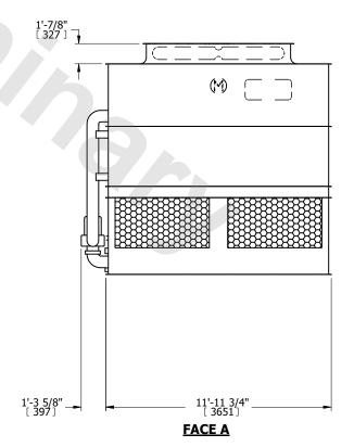
NO. OF SHIPPING SECTIONS **SHIPPING OPERATING** HEAVIEST SECTION 14210 lbs+ [6450] kg+ 12340 lbs+ [5600] kg+ 18380 lbs+ [8340] kg+ WEIGHT WEIGHT WEIGHT
