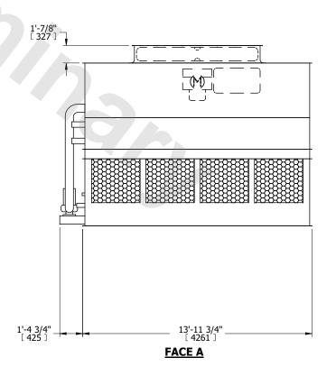
NO. OF SHIPPING SECTIONS **SHIPPING OPERATING** HEAVIEST SECTION 10970 lbs+ [4980] kg+ 15520 lbs+ [7040] kg+ 8890 lbs+ [4035] kg+ WEIGHT WEIGHT WEIGHT
