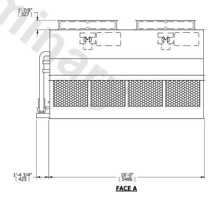
SHIPPING WEIGHT 15030 lbs+ [6820] kg+ OPERATING WEIGHT 20940 lbs+ [9500] kg+ HEAVIEST SECTION WEIGHT 12240 lbs+ [5555] kg+ NO. OF SHIPPING SECTIONS 2 DRAWN BY: JLG
