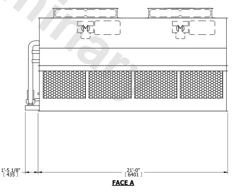
SHIPPING WEIGHT 17240 lbs+ [7820] kg+ OPERATING WEIGHT 24240 lbs+ [11000] kg+ HEAVIEST SECTION WEIGHT 14140 lbs+ [6415] kg+ NO. OF SHIPPING SECTIONS 2 DRAWN BY: JLG
