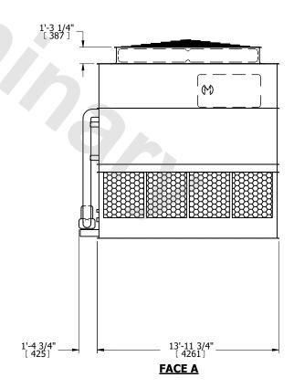
DRAWN BY: NO. OF SHIPPING SECTIONS **SHIPPING** OPERATING HEAVIEST SECTION 19920 lbs+ [9040] kg+ 22980 lbs+ [10425] kg+ 30980 lbs+ [14055] kg+ WEIGHT WEIGHT WEIGHT
