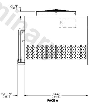
DRAWN BY: SLR NO. OF SHIPPING SECTIONS **SHIPPING** OPERATING HEAVIEST SECTION 29090 lbs+ [13200] kg+ 25170 lbs+ [11420] kg+ 39330 lbs+ [17840] kg+ WEIGHT WEIGHT WEIGHT
