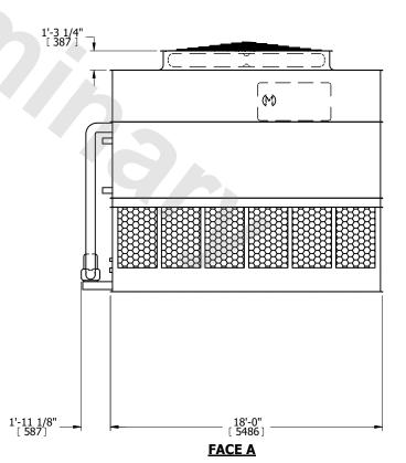
SHIPPING WEIGHT 33900 lbs+ [15380] kg+ OPERATING WEIGHT 44420 lbs+ [20150] kg+ HEAVIEST SECTION WEIGHT 29980 lbs+ [13600] kg+ NO. OF SHIPPING SECTIONS 2 DRAWN BY: SLR
