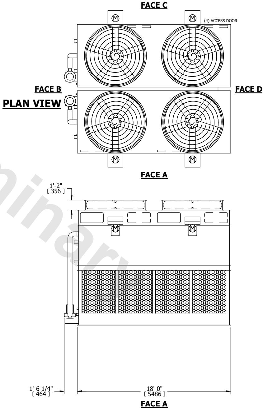
SHIPPING WEIGHT 52920 lbs+ [24005] kg+ OPERATING WEIGHT 57320 lbs+ [26000] kg+ HEAVIEST SECTION WEIGHT 20660 lbs+ [9375] kg+ NO. OF SHIPPING SECTIONS 4 DRAWN BY: TAM
