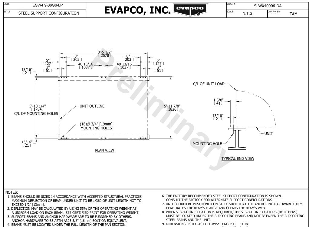
5. SUPPORTING BEAM SURFACE MUST BE LEVEL. DO NOT LEVEL THE UNIT BY PLACING SHIMS BETWEEN THE UNIT MOUNTING FLANGE AND THE SUPPORTING BEAM. [METRIC] [mm]
