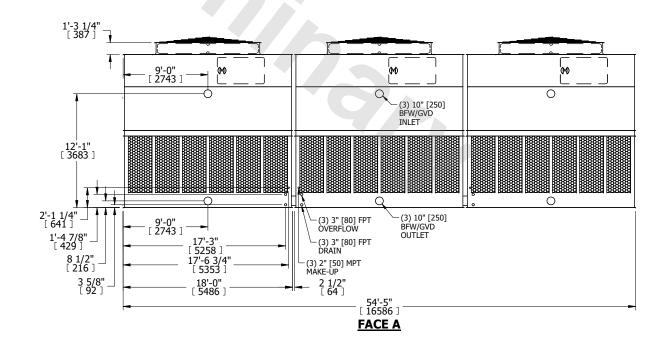
DRAWN BY: KDS NO. OF SHIPPING SECTIONS **SHIPPING** OPERATING HEAVIEST SECTION 35640 lbs+ [16170] kg+ 7700 lbs+ [3495] kg+ 63450 lbs+ [28785] kg+ WEIGHT WEIGHT WEIGHT
