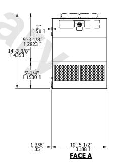
SHIPPING WEIGHT 11340 lbs+ [5145] kg+ OPERATING WEIGHT 17940 lbs+ [8140] kg+ HEAVIEST SECTION WEIGHT 3950 lbs+ [1795] kg+ NO. OF SHIPPING SECTIONS 4 DRAWN BY: KDS
