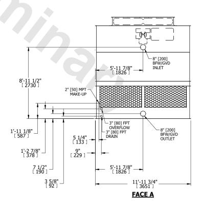
DRAWN BY: JLG NO. OF SHIPPING SECTIONS **SHIPPING** OPERATING HEAVIEST SECTION 5720 lbs+ [2595] kg+ 9580 lbs+ [4350] kg+ 3960 lbs+ [1800] kg+ WEIGHT WEIGHT WEIGHT
