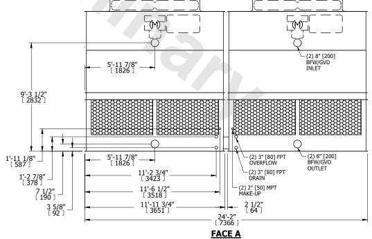
DRAWN BY: JLG OPERATING WEIGHT SHIPPING WEIGHT HEAVIEST SECTION WEIGHT NO. OF SHIPPING SECTIONS 11640 lbs+ [5280] kg+ 19360 lbs+ [8785] kg+ 3960 lbs+ [1800] kg+
