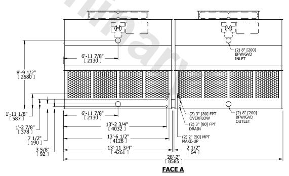
SHIPPING WEIGHT 11980 lbs+ [5435] kg+ OPERATING WEIGHT 21000 lbs+ [9530] kg+ HEAVIEST SECTION WEIGHT 3850 lbs+ [1750] kg+ NO. OF SHIPPING SECTIONS 4 DRAWN BY: JLG
