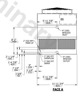
SHIPPING WEIGHT 7500 lbs+ [3405] kg+ OPERATING WEIGHT 13710 lbs+ [6220] kg+ HEAVIEST SECTION WEIGHT 5100 lbs+ [2315] kg+ NO. OF SHIPPING SECTIONS 2 DRAWN BY: KDS
