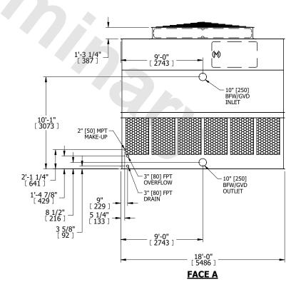
DRAWN BY: KDS NO. OF SHIPPING SECTIONS **SHIPPING** OPERATING HEAVIEST SECTION 11600 lbs+ [5265] kg+ 20870 lbs+ [9470] kg+ 7700 lbs+ [3495] kg+ WEIGHT WEIGHT WEIGHT
