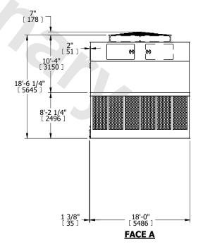
SHIPPING WEIGHT 26500 lbs+ [12025] kg+ OPERATING WEIGHT 45040 lbs+ [20430] kg+ HEAVIEST SECTION WEIGHT 8870 lbs+ [4025] kg+ NO. OF SHIPPING SECTIONS 4 DRAWN BY: KDS
