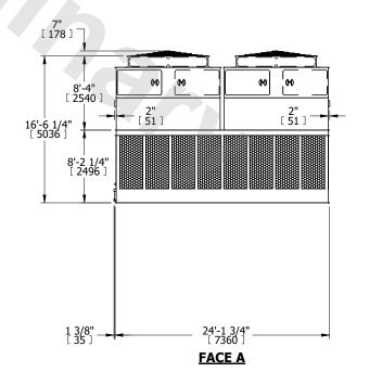
SHIPPING WEIGHT 32380 lbs+ [14690] kg+ OPERATING WEIGHT 56700 lbs+ [25720] kg+ HEAVIEST SECTION WEIGHT 5790 lbs+ [2630] kg+ NO. OF SHIPPING SECTIONS 6 DRAWN BY: JLG
