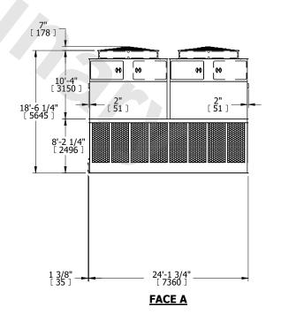
DRAWN BY: JLG NO. OF SHIPPING SECTIONS **SHIPPING OPERATING** HEAVIEST SECTION 35900 lbs+ [16285] kg+ 60220 lbs+ [27320] kg+ 6080 lbs+ [2760] kg+ WEIGHT WEIGHT WEIGHT
