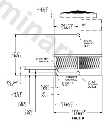
SHIPPING WEIGHT 7790 lbs+ [3535] kg+ OPERATING WEIGHT 12750 lbs+ [5785] kg+ HEAVIEST SECTION WEIGHT 5370 lbs+ [2440] kg+ NO. OF SHIPPING SECTIONS 2 DRAWN BY: JLG
