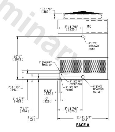
SHIPPING WEIGHT 8040 lbs+ [3650] kg+ OPERATING WEIGHT 13000 lbs+ [5900] kg+ HEAVIEST SECTION WEIGHT 5620 lbs+ [2550] kg+ NO. OF SHIPPING SECTIONS 2 DRAWN BY: JLG
