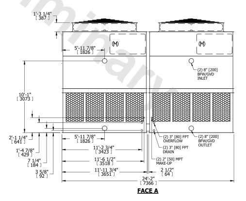
SHIPPING WEIGHT 14580 lbs+ [6615] kg+ OPERATING WEIGHT 24500 lbs+ [11115] kg+ HEAVIEST SECTION WEIGHT 4850 lbs+ [2200] kg+ NO. OF SHIPPING SECTIONS 4 DRAWN BY: KDS
