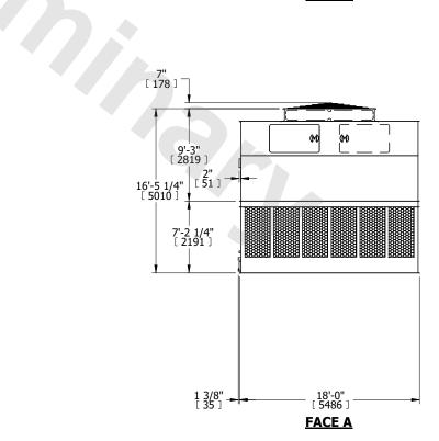
DRAWN BY: JLG NO. OF SHIPPING SECTIONS **SHIPPING** OPERATING HEAVIEST SECTION 20720 lbs+ [9400] kg+ 35920 lbs+ [16295] kg+ 6450 lbs+ [2930] kg+ WEIGHT WEIGHT WEIGHT
