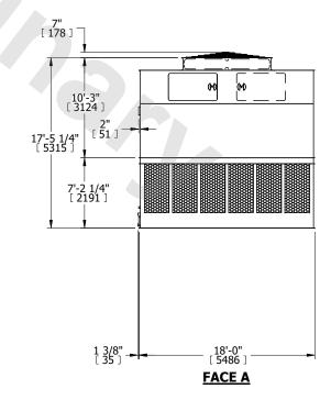
SHIPPING WEIGHT 22780 lbs+ [10335] kg+ OPERATING WEIGHT 37980 lbs+ [17230] kg+ HEAVIEST SECTION WEIGHT 7480 lbs+ [3395] kg+ NO. OF SHIPPING SECTIONS 4 DRAWN BY: KDS
