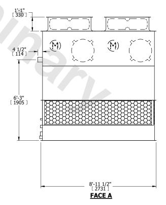
SHIPPING WEIGHT 2100 lbs+ [955] kg+ OPERATING WEIGHT 3650 lbs+ [1660] kg+ HEAVIEST SECTION WEIGHT 1480 lbs+ [675] kg+ NO. OF SHIPPING SECTIONS 2 DRAWN BY: KWC
