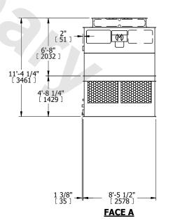
SHIPPING WEIGHT 7240 lbs+ [3285] kg+ OPERATING WEIGHT 12080 lbs+ [5480] kg+ HEAVIEST SECTION WEIGHT 2280 lbs+ [1035] kg+ NO. OF SHIPPING SECTIONS 4 DRAWN BY: JLG
