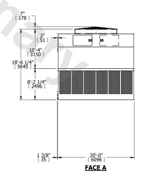
DRAWN BY: KDS NO. OF SHIPPING SECTIONS **SHIPPING** OPERATING HEAVIEST SECTION 28100 lbs+ [12750] kg+ 48900 lbs+ [22185] kg+ 9430 lbs+ [4280] kg+ WEIGHT WEIGHT WEIGHT
