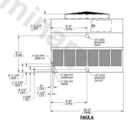
SHIPPING WEIGHT 10660 lbs+ [4840] kg+ OPERATING WEIGHT 19930 lbs+ [9045] kg+ HEAVIEST SECTION WEIGHT 6760 lbs+ [3070] kg+ NO. OF SHIPPING SECTIONS 2 DRAWN BY: KDS
