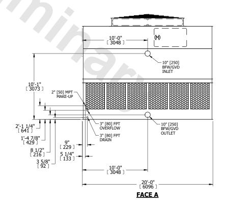
DRAWN BY: KDS NO. OF SHIPPING SECTIONS **SHIPPING** OPERATING HEAVIEST SECTION 12470 lbs+ [5660] kg+ 22870 lbs+ [10375] kg+ 8360 lbs+ [3795] kg+ WEIGHT WEIGHT WEIGHT
