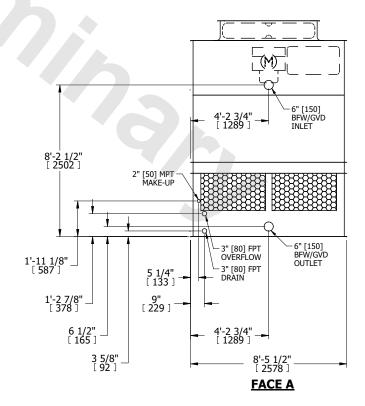
SHIPPING WEIGHT 3340 lbs+ [1515] kg+ OPERATING WEIGHT 5380 lbs+ [2445] kg+ HEAVIEST SECTION WEIGHT 2210 lbs+ [1005] kg+ NO. OF SHIPPING SECTIONS
