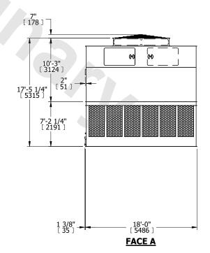
SHIPPING WEIGHT 21740 lbs+ [9865] kg+ OPERATING WEIGHT 36940 lbs+ [16760] kg+ HEAVIEST SECTION WEIGHT 6960 lbs+ [3160] kg+ NO. OF SHIPPING SECTIONS 4 DRAWN BY: KDS
