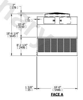
DRAWN BY: KDS NO. OF SHIPPING SECTIONS **SHIPPING** OPERATING HEAVIEST SECTION 25420 lbs+ [11535] kg+ 43960 lbs+ [19940] kg+ 8330 lbs+ [3780] kg+ WEIGHT WEIGHT WEIGHT
