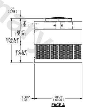
DRAWN BY: KDS NO. OF SHIPPING SECTIONS **SHIPPING** OPERATING HEAVIEST SECTION 27240 lbs+ [12360] kg+ 9000 lbs+ [4085] kg+ 48040 lbs+ [21795] kg+ WEIGHT WEIGHT WEIGHT
