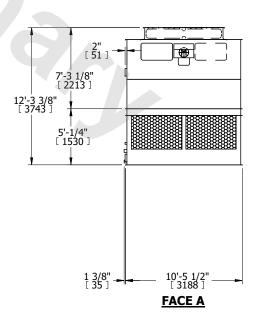
SHIPPING WEIGHT 9700 lbs+ [4400] kg+ OPERATING WEIGHT 16300 lbs+ [7395] kg+ HEAVIEST SECTION WEIGHT 3130 lbs+ [1420] kg+ NO. OF SHIPPING SECTIONS 4 DRAWN BY: JLG
