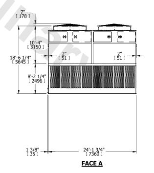
DRAWN BY: JLG NO. OF SHIPPING SECTIONS **SHIPPING** OPERATING HEAVIEST SECTION 36500 lbs+ [16560] kg+ 60820 lbs+ [27590] kg+ 6230 lbs+ [2830] kg+ WEIGHT WEIGHT WEIGHT
