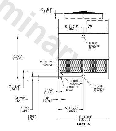
SHIPPING WEIGHT 7520 lbs+ [3415] kg+ OPERATING WEIGHT 12480 lbs+ [5665] kg+ HEAVIEST SECTION WEIGHT 5100 lbs+ [2315] kg+ NO. OF SHIPPING SECTIONS 2 DRAWN BY: JLG
