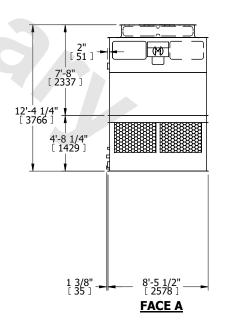
SHIPPING WEIGHT 7660 lbs+ [3475] kg+ OPERATING WEIGHT 12500 lbs+ [5670] kg+ HEAVIEST SECTION WEIGHT 2490 lbs+ [1130] kg+ NO. OF SHIPPING SECTIONS 4 DRAWN BY: JLG
