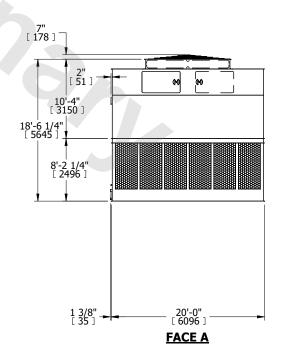
DRAWN BY: KDS NO. OF SHIPPING SECTIONS **SHIPPING** OPERATING HEAVIEST SECTION 26920 lbs+ [12215] kg+ 8840 lbs+ [4010] kg+ 47720 lbs+ [21650] kg+ WEIGHT WEIGHT WEIGHT
