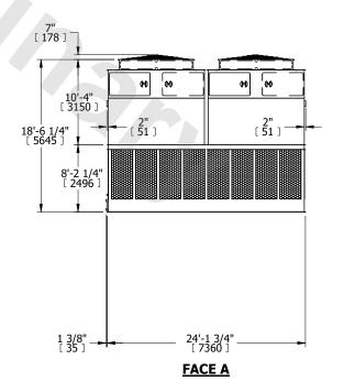
DRAWN BY: JLG NO. OF SHIPPING SECTIONS **SHIPPING** OPERATING HEAVIEST SECTION 35140 lbs+ [15940] kg+ 59460 lbs+ [26975] kg+ 5890 lbs+ [2675] kg+ WEIGHT WEIGHT WEIGHT
