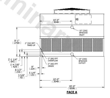
DRAWN BY: KDS NO. OF SHIPPING SECTIONS **SHIPPING** OPERATING HEAVIEST SECTION 11370 lbs+ [5160] kg+ 21770 lbs+ [9875] kg+ 7260 lbs+ [3295] kg+ WEIGHT WEIGHT WEIGHT
