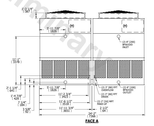
SHIPPING WEIGHT 15080 lbs+ [6845] kg+ OPERATING WEIGHT 25000 lbs+ [11340] kg+ HEAVIEST SECTION WEIGHT 5100 lbs+ [2315] kg+ NO. OF SHIPPING SECTIONS 4 DRAWN BY:
