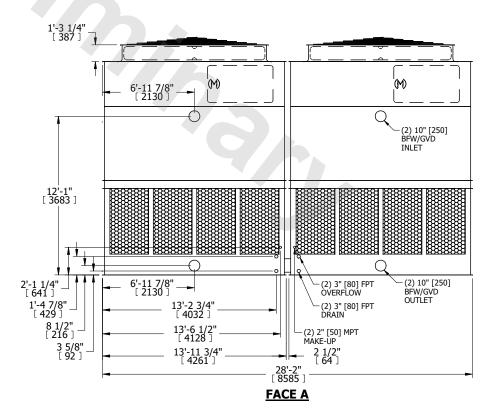
SHIPPING WEIGHT 19320 lbs+ [8765] kg+ OPERATING WEIGHT 33980 lbs+ [15415] kg+ HEAVIEST SECTION WEIGHT 6610 lbs+ [3000] kg+ NO. OF SHIPPING SECTIONS 4 DRAWN BY: KDS
