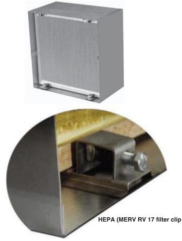
Some applications will have a three filter system, a pre, an intermediate and a final filter. The pre and intermediate filters are held in the same pre- filter frame at the inlet of the unit using the same type of "P" clip, only longer to accommodate the intermediate filter frame. The intermediate filter "pushes through" the frame and the pre filters sits in front. The following shows the installation of the "P" clip. Four clips are used with a pre and intermediate filter installation.
