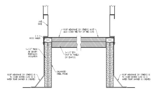
Roof Mounting curb detail for lower temperature applications (see specific job order I for curb detail)
