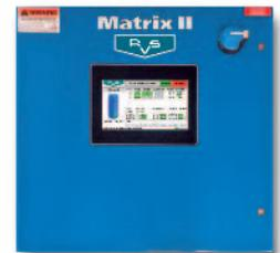
**MMP-C (Charlie):** Medium standard enclosure panel for up to three pumps plus one transfer pump maximum with starters and disconnect, one I/O board, with color graphic HMI touch screen display mounted in the enclosure door, 24"W x 36"H x 10"D enclosure dimensions.
