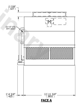
DRAWN BY: JLG NO. OF SHIPPING SECTIONS **SHIPPING OPERATING** HEAVIEST SECTION 14310 lbs+ [6495] kg+ 20300 lbs+ [9210] kg+ 12440 lbs+ [5645] kg+ WEIGHT WEIGHT WEIGHT
