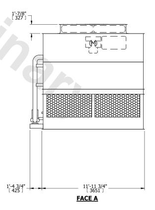
SHIPPING WEIGHT 14070 lbs+ [6385] kg+ OPERATING WEIGHT 18240 lbs+ [8275] kg+ HEAVIEST SECTION WEIGHT 12200 lbs+ [5535] kg+ NO. OF SHIPPING SECTIONS 2 DRAWN BY: JLG
