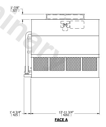
DRAWN BY: JLG NO. OF SHIPPING SECTIONS **SHIPPING** OPERATING HEAVIEST SECTION 18760 lbs+ [8510] kg+ 16680 lbs+ [7570] kg+ 23750 lbs+ [10775] kg+ WEIGHT WEIGHT WEIGHT
