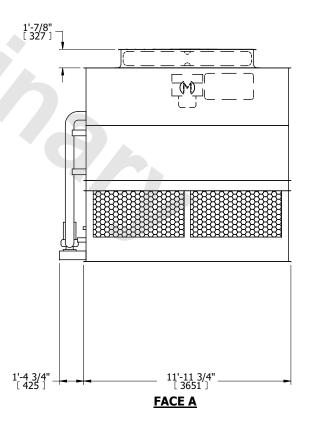
DRAWN BY: JLG NO. OF SHIPPING SECTIONS **SHIPPING OPERATING** HEAVIEST SECTION 14210 lbs+ [6450] kg+ 18380 lbs+ [8340] kg+ 12340 lbs+ [5600] kg+ WEIGHT WEIGHT WEIGHT
